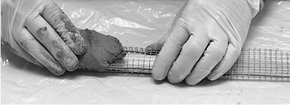
Apply a smooth concrete to the small mesh form by pushing it well into the wire to completely cover and surround it (1). The foam core stops the mix from being pushed to the other side. On the blade part you must use your own fingers to stop the mix from being pushed through.
