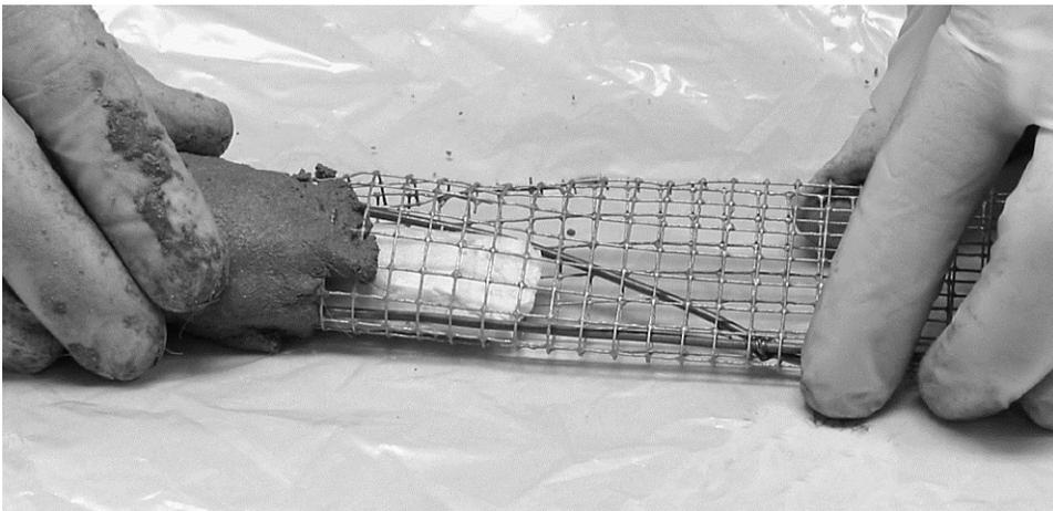
More detail (2) showing the mesh, the steel rod, foam, and the concrete pushed into place. Try and cover all the wire in this first step.
